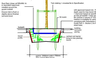
SITE ROAD TREE PLANTING TRENCH FOR NEW EHS (up to 18-20cm) TREES SHOWING ROOT BARRIER, STAKING AND ROOT AERATION DRAIN
